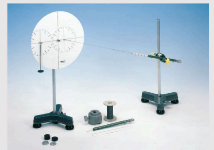
Fig.1: Experimental set-up for investigating moments in equilibrium.
